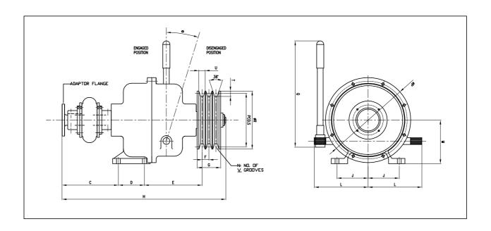
$\label{lem:machweld-Engineers-Marine-Power-Take-Offs. are manufactured to cater marine sector. This application is widely used as front Power Take-Off to drive the winch on fishing boats.$
